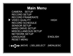
Video Quality can be set to Highest, High, Normal, and Low. The higher settings produce better images, but use up more hard drive space. The cameras are all set to the same setting in one step in the Main Menu.
